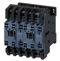
Reversing contactor assembly AC-3,18 kW/400 V,AC230V,50/60Hz 3-pole, Size S0 Spring-type terminal electrical and mechanical Interlock 2 NO integrated
