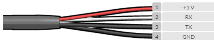
Communication cable pinout
