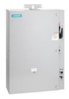
Pump control panel, Size 3 1/2, Three phase full voltage, Solid-state overload relay, OLR amp range 50-200A, 208VAC 60Hz coil, Standard type contactor, 200A fusible disconnect, 200A/250V fuse clip, HOA Sel Sw. <(>&<)> Start P.B., Enclosure NEMA type 3/3R, Weather proof outdoor use
