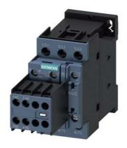
Contactor, AC-3, 18.5 kW / 400 V, 2 NO + 2 NC, 110 V AC, 50 Hz, 3-pole, Size S0 Screw terminal Removable auxiliary switch
