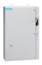
Non-reversing motor starter, Size 3, Three phase full voltage, Solid-state overload relay, OLR amp range 25-100A, 110V 50Hz / 120V 60Hz coil, Combination type, 100A fusible disconnect, 100A/250V fuse clip, Enclosure NEMA type 4/12, Water/dust tight for outdoors, Extra-wide enclosure
