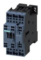
Power contactor, AC-3 25 A, 11 kW / 400 V 2 NO + 2 NC 24 V DC 4-pole size S0 Spring-type terminals 1 NO + 1 NC integrated
