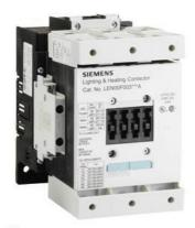
Electrically held lighting contactor, Contactor amp rating 200A, 0 N.C. / 3 N.O. Poles, 110VAC 50HZ/120VAC 60HZ coil, Non-combination type, (no disconnect device), Enclosure NEMA type (open), No enclosure
