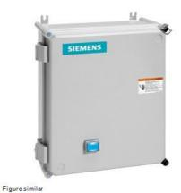
Non-reversing motor starter, Size 3 1/2, Three phase full voltage, Amb. compensate bimetal OLR, Contactor amp rating 115A, 24VDC coil, Non-combination type, Enclosure type 4X fiberglass, Water/dust tight noncorrosive
