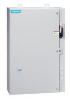
Non-reversing motor starter, Size 2 1/2, Three phase full voltage, Solidstate overload relay, OLR amp range 25-100A, Combination type, 100A fusible disconnect, 100A/600V fuse clip, Enclosure NEMA type 4/12, Water/dust tight for outdoors, Extra-wide enclosure
