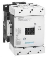
Electrically held lighting contactor, Contactor amp rating 400A, 0 N.C. / 3 N.O. Poles, 110VAC 50HZ/120VAC 60HZ coil, Non-combination type, (no disconnect device), Enclosure NEMA type (open), No enclosure
