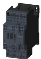
power contactor, AC-3 25 A, 11 kW / 400 V 1 NO + 1 NC, 24 V AC, 50 / 60 Hz, 3-pole, Size S0, Spring-type terminal
