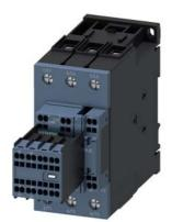
Traction contactor, AC-3 80 A, 37 kW / 400 V 2 NO + 2 NC 110 V DC, 0.7-1.25\* Us with varistor 3-pole, size S2 Spring-type terminals
