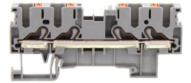
Feed-through terminal, Push-in connection, Mounting type: Mounting rail TS 35/7.5, Rated cross-section: 4 mm<sup>2</sup>, Width: 6.1 mm, Colour: Grey
