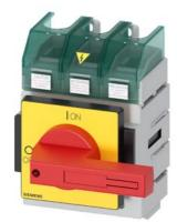
SENTRON, Molded case switch 3LD5 UL, Emergency switching-off, 3-pole, certified according to UL489 UL60947-4-1 and IEC60947-3, UL: 150A, SCCR 50kA at 480VAC, Operating power at 480VAC 3-phase: 100hp, IEC: 160A, Operating power at AC-23A at 400V: 75kW, floor mounting with direct handle, red/yellow, incl. terminal covers for the infeed side
