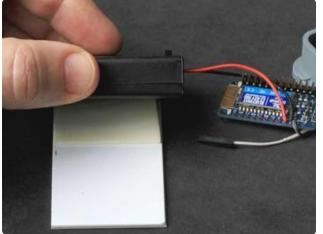
Remove the backing and attach the battery box.
