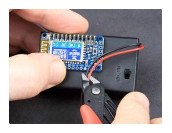
Position the EZ-Key on top of the battery holder as shown. Measure and cut the wires so they are just long enough to reach the Vin and Gnd holes on the board.
