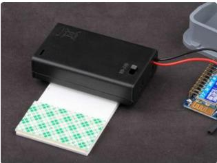
Cut another piece of tape and attach to the other end of the plastic plate.
