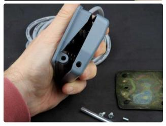
Push on the end of the hinge-pin with the tip of the screwdriver. While squeezing the foot switch, pull the hinge pin completely out.
