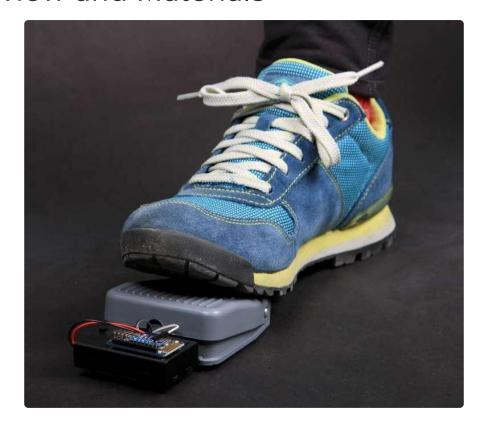
This is a quick and easy project that will be speed your work on future projects. By combining an Adafruit BlueFruit EZ-Key with a foot switch, we end up with a wireless, hands-free scroll button. No need to put down that hot iron to see the next step in the tutorial. Just give the pedal a tap with your foot to scroll down the page.
