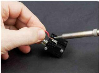
Remove the switch and use a soldering iron to de-solder the old wires.
