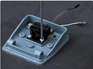
Feed the ends of the jumpers through the cable hole and re-install the switch.
