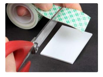
Cut a piece of double-sided foam tape about as wide as the plastic plate (1 3/4") and stick to one end of the plate.
