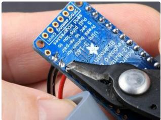
Solder one of the wires from the switch to one of the other Gnd holes, and clip the soldered wires close to the board.
