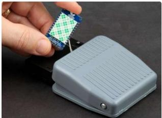
Cut another piece of tape to fit on the bottom side of the EZ-Key. Mount the EZ-Key to the top of the battery box. Keep to the left so you don't cover the ON/OFF switch.
