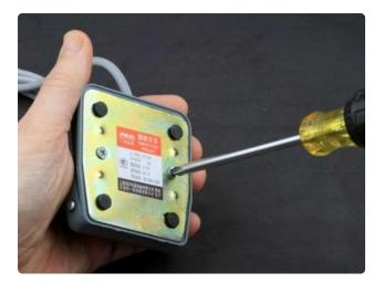
Remove the two screws from the bottom of the foot switch. Remove the bottom plate being careful to keep the bottom of the switch facing up.
