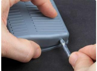
Press down on the top half of the switch to align the holes and insert the hinge pin.
