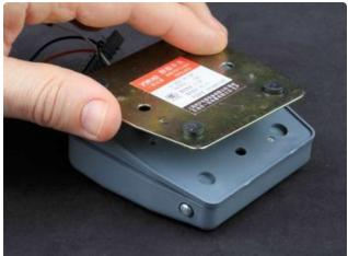
Re-install the locking pin and replace the bottom cover.
