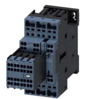
Power contactor, AC-3 38 A, 18.5 kW / 400 V 2 NO + 2 NC, 230 V AC 50 Hz, 3-pole, size S0 Spring-type terminals Removable auxiliary switch
