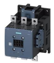
power contactor, AC-3 225 A, 110 kW / 400 V AC (50-60 Hz) / DC operation 110-127 V AC/DC auxiliary contacts 2 NO + 2 NC 3-pole, frame size S10 busbar connections drive: conventional screw terminal
