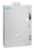
Pump control panel, Size 3, Three phase full voltage, Solid-state overload relay, OLR amp range 25-100A, 380-440/440-480V 50/60Hz coil, Standard type contactor, 200A fusible disconnect, 200A/600V fuse clip, HOA Sel Sw. <(>&<)> Start P.B., Enclosure NEMA type 3/3R, Weather proof outdoor use
