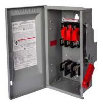
Siemens Low Voltage Circuit Protection Heavy Duty Safety Switches. Type: ENCLOSED, SAFETY SWITCH Std: CUL V. Rating: 600V A. Rating: 60A Wattage: 6W No. Of Poles: 6P F. Rating: 60Hz Action: SINGLE THROW Material: 304SS Enclosure: TYPE 3R/12. 2-3 point mounting holes. Insulation: YES O. Cycles: 10000 O. Temperature: (-20F-120F) AMBIENT TEMPERATURE Environmental Conditions: OUTDOOR/INDUSTRIAL
