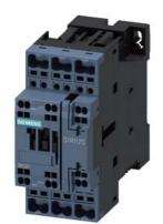
Traction contactor, AC-3 32 A, 15 kW / 400 V 1 NO + 1 NC with solid-state operating mechanism 72 V DC, 0.7-1.25\*Us with integrated varistor 3-pole, size S0 Spring-type terminals
