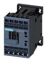
power contactor, AC-3 12 A, 5.5 kW / 400 V 1 NC, 220 V DC 3-pole, Size S00 Spring-type terminal
