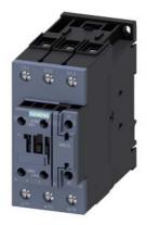
power contactor, AC-3 51 A, 22 kW / 400 V 1 NO + 1 NC, 208 V AC, 50 / 60 Hz, 3-pole, size S2, screw terminal
