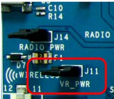
Figure 5-29. CY8CKIT-001 PSoC DVK VR_POWER Jumper
