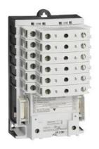
Electrically held lighting contactor, (convertible to mech. held), Amp rating 30A (tungsten 20A), 7 N.C. / 0 N.O. poles, 24V 60Hz / 20V 50Hz coil, Noncombination type, Enclosure NEMA type (open), No enclosure
