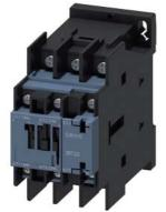
power contactor, AC-3 12 A, 5.5 kW / 400 V 1 NO + 1 NC, 100 V AC, 50 Hz 100-110 V, 60 Hz, 3-pole Size S0 ring cable lug connection
