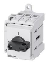
Load disconnector 3LD3, lu 63 A Main switch 3-pole Rated operating capacity at AC-23 A at 400V 22.0 kW Installation in distribution boards, Basic switch with selector knob black with auxiliary switch 1OE + 1S
