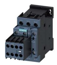
Power contactor, AC-3 38 A, 18.5 kW / 400 V 2 NO + 2 NC, 24 V AC 50/60 Hz, 3-pole Size S0, screw terminals Removable auxiliary switch
