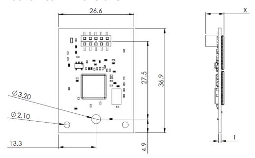
All dimensions in mm. Tolerance on all dimensions ± 0.5mm.
