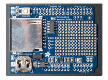
This is the older Datalogger shield. In particular, note that the prototyping area is completely full of 0.1" spaced holes
