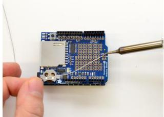
Place the board on the Metro and solder the 2x3 header
