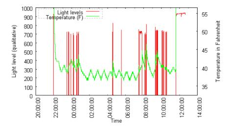
You can see in the middle and end the temp and light levels are very high because the logger was outside the fridge. The green line is the temperature so you can see the temperature slowly rising and then the compressor kicking in every half hour or so. The red lines indicate when the door was opened. This night was a more insominac one than normal!
