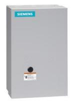
Mechanically held lighting contactor, Contactor amp rating 100A, 0 N.C. / 5 N.O. poles, 440VAC 50HZ/480VAC 60HZ coil, Non-combination type, Enclosure NEMA type 1, Indoor general purpose use
