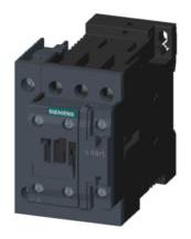
Contactor, AC-1, 35 A/400 V/40  $^{\circ}\text{C}$  , S0, 4-pole, 48 V DC, 1 NO+1 NC, screw terminal
