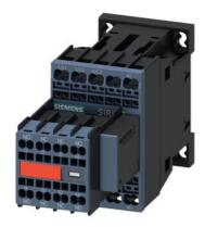
Power contactor, AC-3 7 A, 3 kW / 400 V 2 NO + 2 NC, 110 V AC, 50 Hz 120 V, 60 Hz, with plugged-on varistor, 3-pole, Size S00, Spring type terminal Captive auxiliary switch
