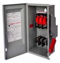
Siemens Low Voltage Circuit Protection Heavy Duty Safety Switch. 3-Pole 3-Fuse and solid neutral Fused in a type 1 enclosure (indoor). Rated 240VAC (200A).
