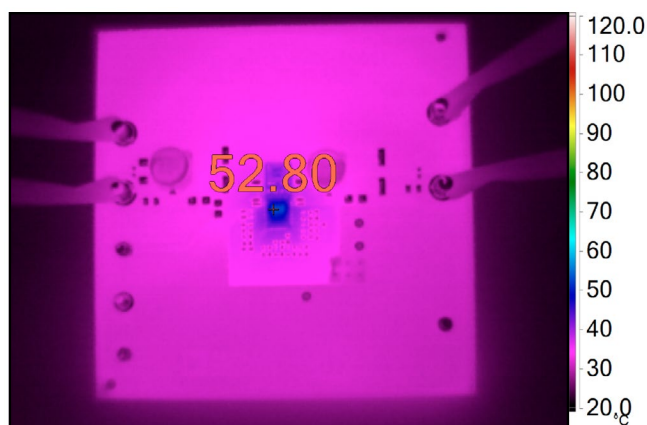
Figure 6. DC3103A Thermal Image, 10 Minute Runtime, 23°C Ambient PV_{IN} = 12V , V_{OUT} = 12V , I_{OUT} = 1A , SSFM OFF
