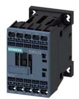
Power contactor, AC-3 16 A, 7.5 kW / 400 V 1 NC, 60 V DC 3-pole, Size S00 Spring-type terminals
