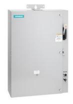
Pump control panel, Size 3 1/2, Three phase full voltage, Solid-state overload relay, OLR amp range 50-200A, 110V 50Hz / 120V 60Hz coil, Standard type contactor, 200A fusible disconnect, 200A/250V fuse clip, HOA Sel Sw. <(>&<)> Start P.B., Enclosure NEMA type 3/3R, Weather proof outdoor use
