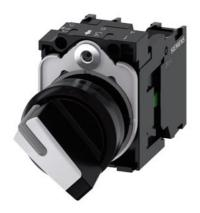
Selector switch, illuminable, 22 mm, round, plastic, white, selector switch, short, 2 switch positions O-I, latching, 10:30h/13:30h, with holder, 1 NO, 1 NC, screw terminal, with laser labeling, upper case
