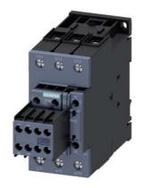
power contactor, AC-3 40 A, 18.5 kW / 400 V 2 NO + 2 NC, 230 V AC 50 Hz, 3-pole, Size S2, screw terminal
