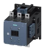
power contactor, AC-3 400 A, 200 kW / 400 V AC (50-60 Hz) / DC operation 110-127 V AC/DC auxiliary contacts 2 NO + 2 NC 3-pole, frame size S12 busbar connections drive: conventional spring-loaded terminal
