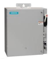
Pump control panel, Size 5, Three phase full voltage, Solid-state overload relay, OLR amp range 55-250A, 220-240V 50-60Hz/DC coil, Standard type contactor, 250A circuit breaker, HOA Sel Sw. <(>&<)> Start P.B., Enclosure NEMA type 3/3R, Weather proof outdoor use
