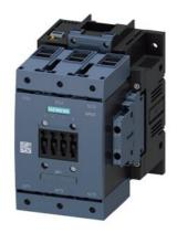
power contactor, AC-3 115 A, 55 kW / 400 V AC (50-60 Hz) / DC operation 96-127 V AC/DC auxiliary contacts 2 NO + 2 NC 3-pole, frame size S6 with box terminals drive: electronic with PLC interface 24 V DC screw terminal
