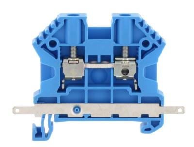
Feed-through terminal, Screw connection, Mounting type: Mounting rail TS 35/7.5, Rated cross-section: 4 mm², Width: 6 mm, Colour: Blue
