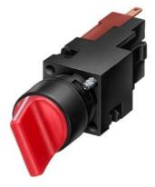
Selector switch, 16 mm, round, plastic, black, 2 switch positions O-I, latching, actuating angle 62 degree, 1 NO  $\,$
