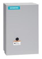
Electrically held lighting contactor, Contactor amp rating 30A, 0 N.C. / 12 N.O. Poles, 24VAC 50/60HZ coil, Non-combination type, (no disconnect device), Enclosure NEMA type 1, Indoor general purpose use
