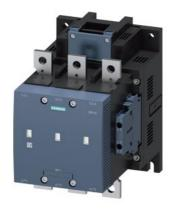
vacuum contactor, AC-3 265 A, 132 kW / 400 V AC (50-60 Hz) / DC operation 23-26 V AC/DC auxiliary contacts 2 NO + 2 NC 3-pole, frame size S10 busbar connections drive: conventional
