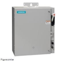
Pump control panel, Size 3, Three phase full voltage, Solid-state overload relay, OLR amp range 25-100A, 220-240/440-480VAC 60Hz coil, Standard type contactor, 100A circuit breaker, HOA Sel Sw. <(>&<)> Start P.B., Enclosure NEMA type 3/3R, Weather proof outdoor use
