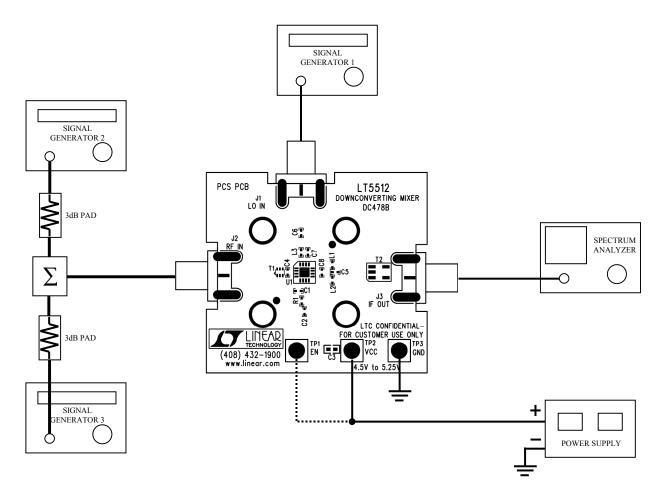
Figure 3. Test Set-Up for Mixer Two-Tone Measurements.
