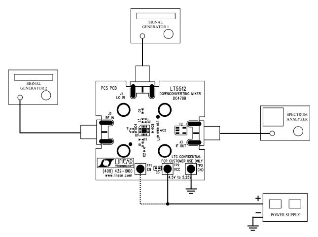
Figure 2. Test Set-Up for Mixer Single-Tone Measurements.
