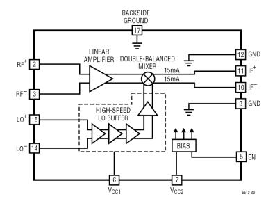
Figure 1. LT5512 IC Block Diagram
