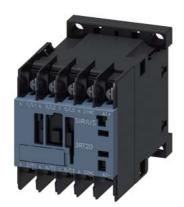
Power contactor, AC-3 16 A, 7.5 kW / 400 V 1 NC, 24 V DC 3-pole, Size S00 ring cable lug connection
