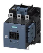
power contactor, AC-3 185 A, 90 kW / 400 V AC (50-60 Hz) / DC operation 200-277 V AC/DC auxiliary contacts 2 NO + 2 NC 3-pole, frame size S6 busbar connections drive: electronic with PLC interface 24 V DC spring-loaded terminal
