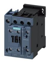
Contactor, AC-1, 40 A/400 V/40 °C, S0, 4-pole, 208 V AC, 50/60 Hz, 1 NO+1 NC, screw terminal
